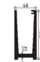
Continuous Railing Bottom Section Number: V-10003 Weight (kg/12'): 14.875
