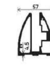
Continuous Railing Bottom Section Number: V-10002 Weight (kg/12'): 9.100
